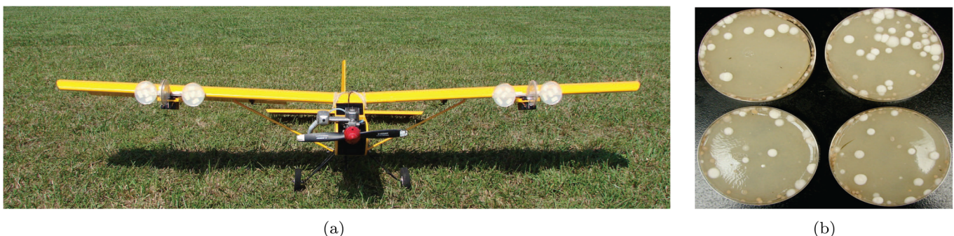
FIG. 3. (Color online) An autonomous UAV equipped with microbe-sampling devices for collecting Fusarium in the lower atmosphere (a). The sampling devices are closed during takeoff and landing and are opened once the UAV has reached its target sampling altitude. Petri plates with white colonies of Fusarium cultured from an individual sampling mission are shown in (b).
