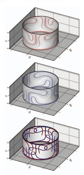
FIG. 5. (Color) FTLE on a cylinder for a positive integration time (upper panel) and a negative integration time (middle panel). Corresponding attractive and repulsive LCS (lower panel) (enhanced online). [URL: http://dx.doi.org/10.1063/1.3278516.1]
