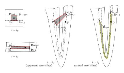
FIG. 3. (Color online) Using elements that are too large can lead to an underestimated FTLE. Starting with a square element at  $t=t_0$ , the stretching is well captured by the motion of the four grid points at a later time  $t=t_1$ . Nevertheless, the deformation is nonlinear and the element can fold at a later time  $t=t_f$ . At this time, the algorithm that uses the position of the four grid points to evaluate FTLE will underestimate the actual stretching
