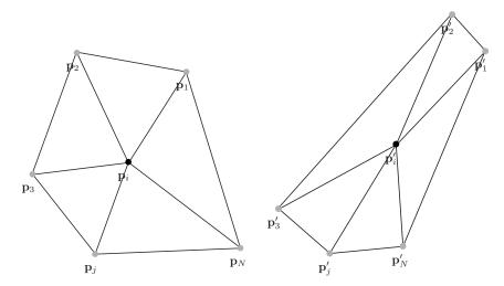
FIG. 2. Deformation of an unstructured mesh under the flow. Left panel: the node  $\mathbf{p}_i$  has N neighbors  $\mathbf{p}_1$ ,  $\mathbf{p}_2,\ldots,\mathbf{p}_j,\ldots,\mathbf{p}_N$ . Right panel: under the action of the flow, the node  $\mathbf{p}_i$  moves to the position  $\mathbf{p}_i'$ . The deformed edges  $\mathbf{p}_1'-\mathbf{p}_i',\mathbf{p}_2'-\mathbf{p}_i',\ldots,\mathbf{p}_j'-\mathbf{p}_i',\ldots,\mathbf{p}_N'-\mathbf{p}_i'$  are used to approximate the deformation tensor.
